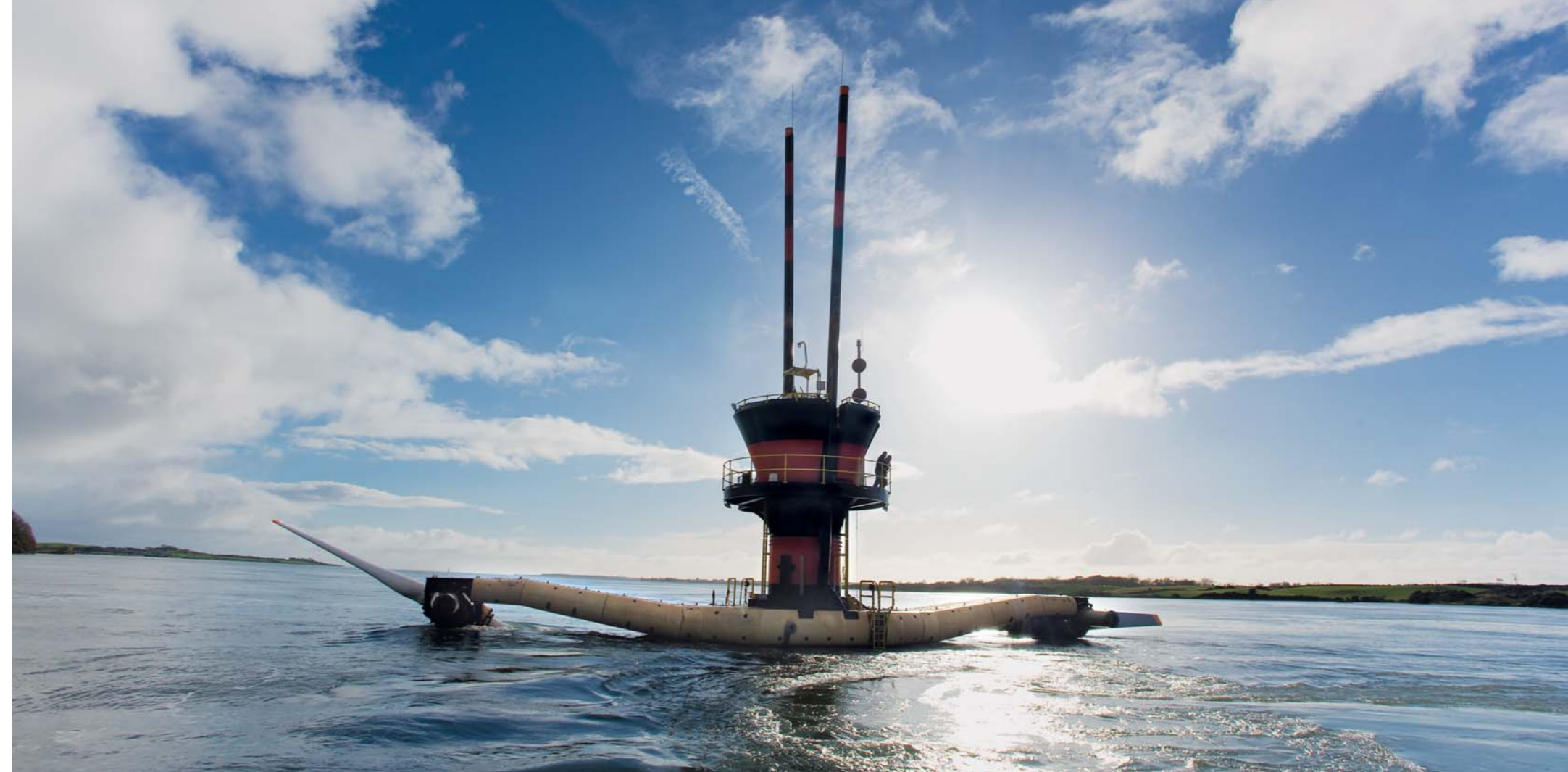
Harnessing tidal power in Northern Ireland’s Strangford Lough: At 1.2 MW, SeaGen is the world’s first commercial-scale tidal turbine.
