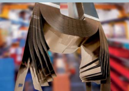
Transformers with amorphous steel cores have very low no-load operation losses.
