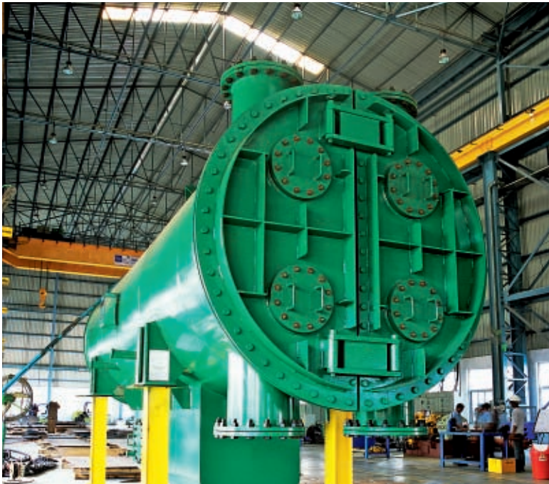
Steam-turbine (top) and condenser manufacturing (bottom) at Siemens' Vadodara plant, India.
