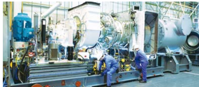
SGT-400 compressor package assembly.
