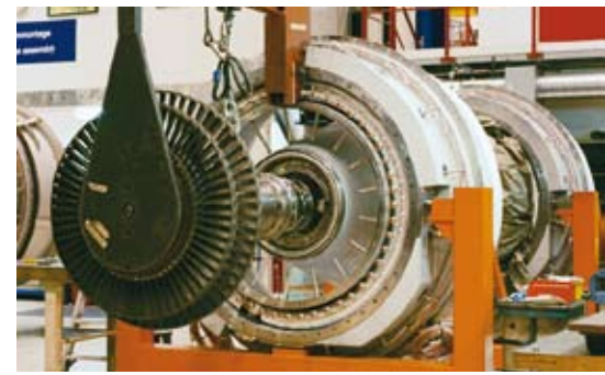
SGT-600 power-turbine rotor-assembly.
