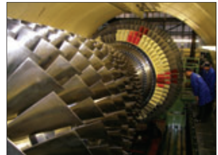
Abb. 5: SGT5-8000H – 13-stufiger Axialverdichter.
