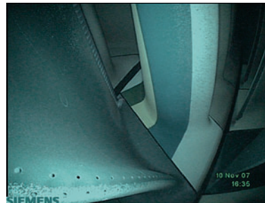
Blade 2 with thermal paint and identification stripes after test run
