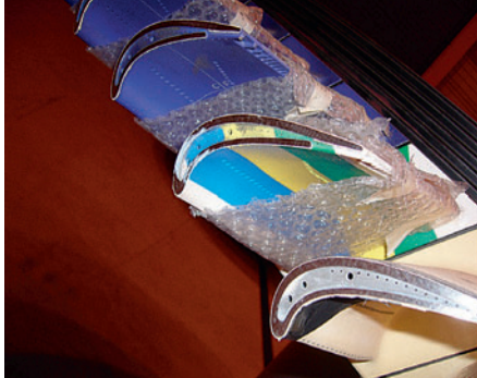
Blade 1: Prepared for measurements and with stripes for identification during operation
