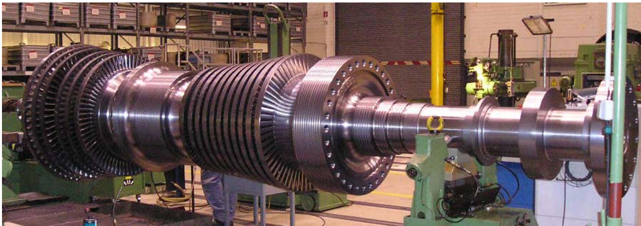
Figure 8 – BB44FA Fully Assembled HP/IP Rotor
