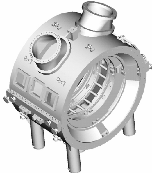
Figure 15 - Inner Casing Solid Model
