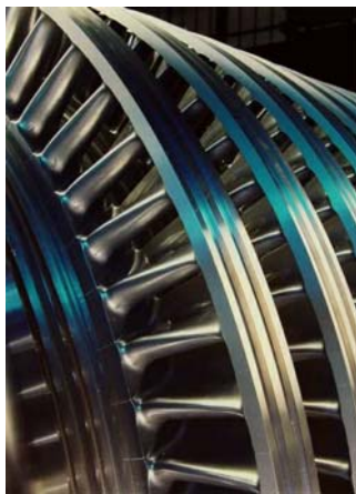
Figure 9 – Integrally Shrouded Tee-Root Blade
