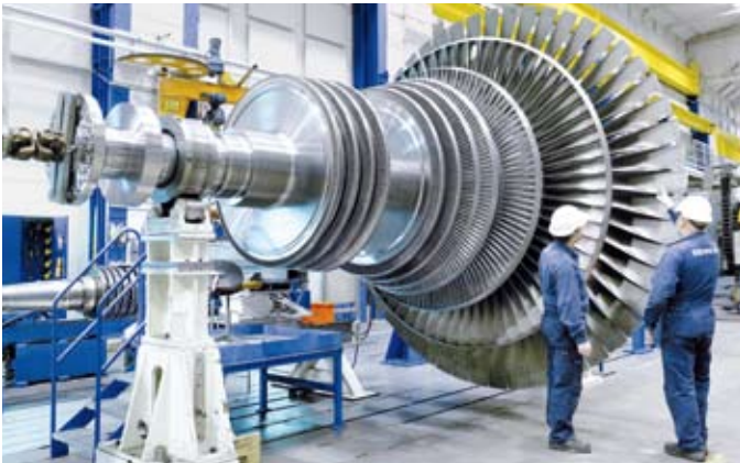
Final rotor assembly for the SST-700 to serve in the Amsterdam Waste-to-Heat facility
