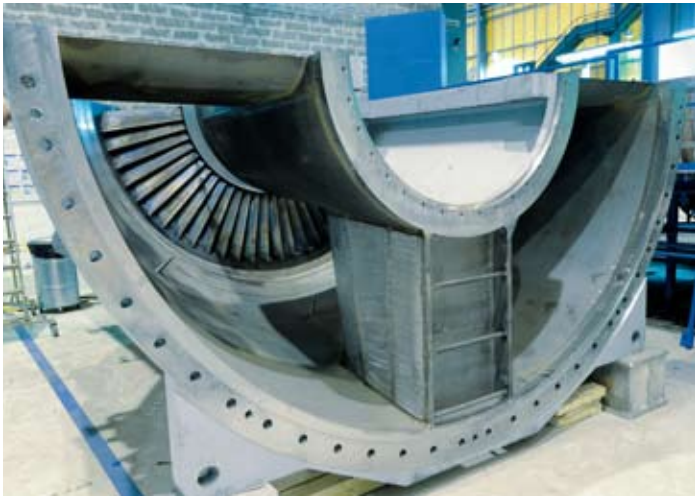
SST-700 LP module for the Andasol CSP plant in Spain.
