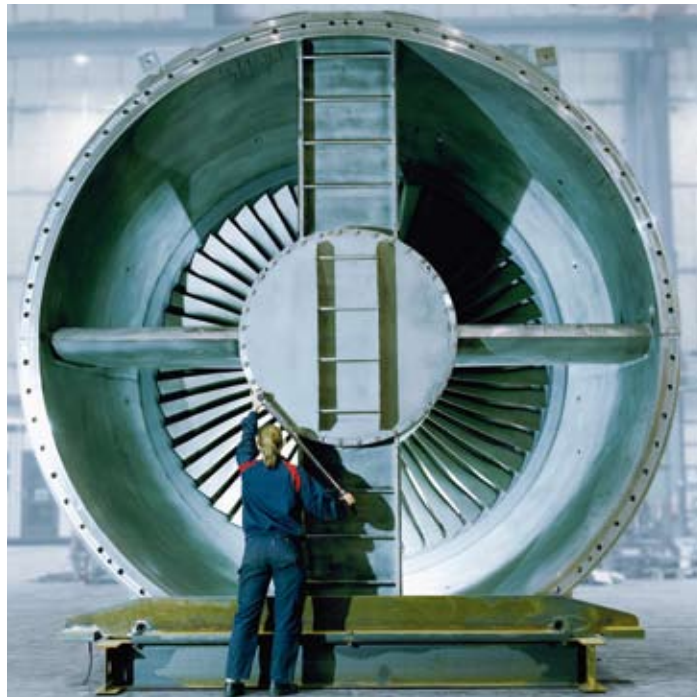
Axial exhaust of a SST-900 steam turbine.
