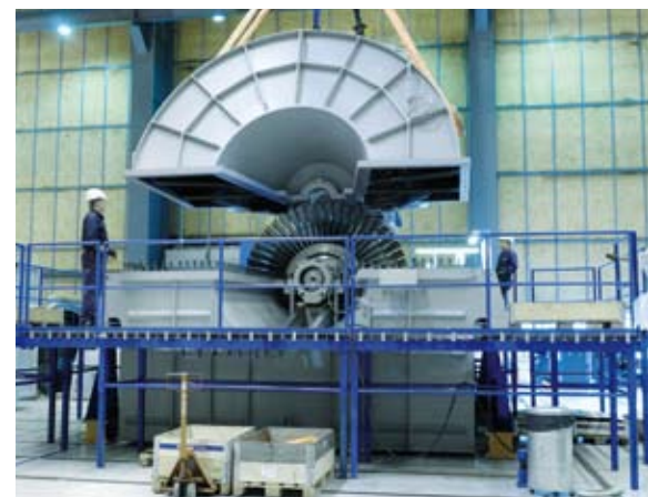
SST-900 steam turbine in the workshop in Finspong, Sweden.
