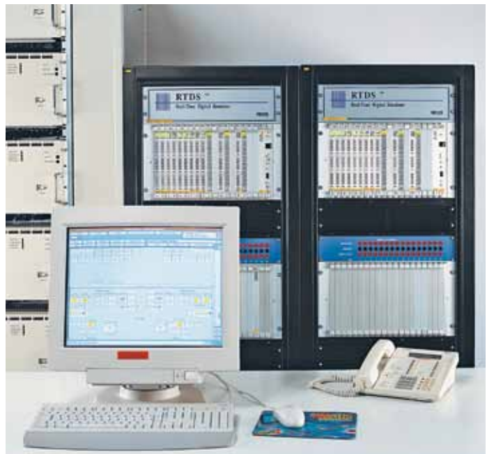
Fig. 5.7: All controls are fully tested with a real-time digital simulator
