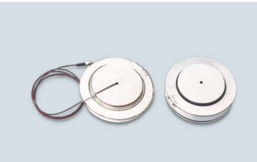
Fig. 7.1: Easily assembled direct light triggered thyristors (left) have prevailed over electrically triggered models (ETT, right), especially in high-voltage thyristor valves
