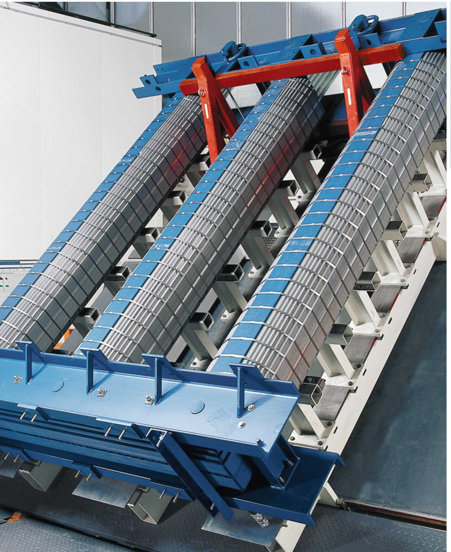
Fast and precise stacking of core laminations on special stands: The joints are step-lapped. The best way to keep noise and losses low.
