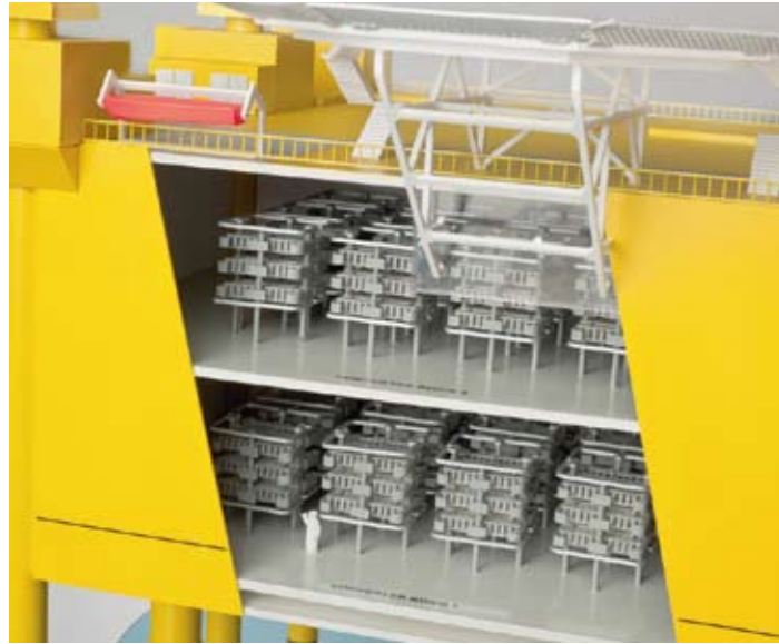
A model of Siemens' wind power offshore substation (WIPOS): Siemens supplies comprehensive offshore grid connection solutions with flexible substation configurations for both AC and DC applications.
