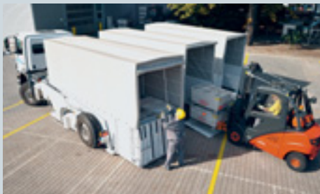
Logistics challenge: Interchangeable swap bodies are used for internal blade transport to save valuable time.
