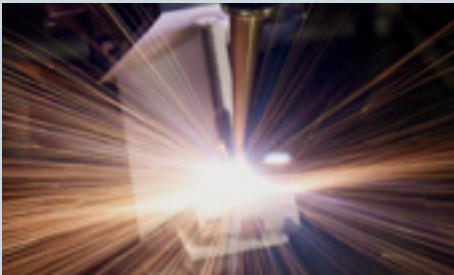
Cutting of cooling air holes using a highly innovative laser process ensures that the blades do not overheat in operation.
