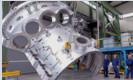
A section of the casing shortly before assembly. Weighing 25 metric tons, it forms part of the largest and most powerful gas turbine in the world.
