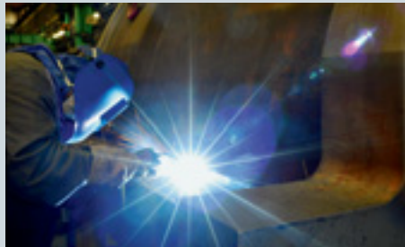
Worker safety is extremely important at the gas turbine factory, as in this example of welding work on the turbine casing.
