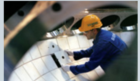
Siemens holds 15 patents on its ceramic heat shields, which are unique worldwide in terms of functionality and stressing capability.
