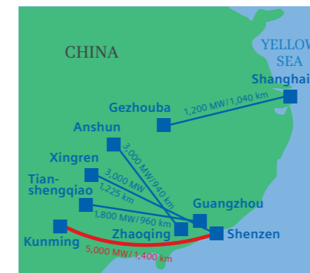
Sharing power in China: HVDC systems.
