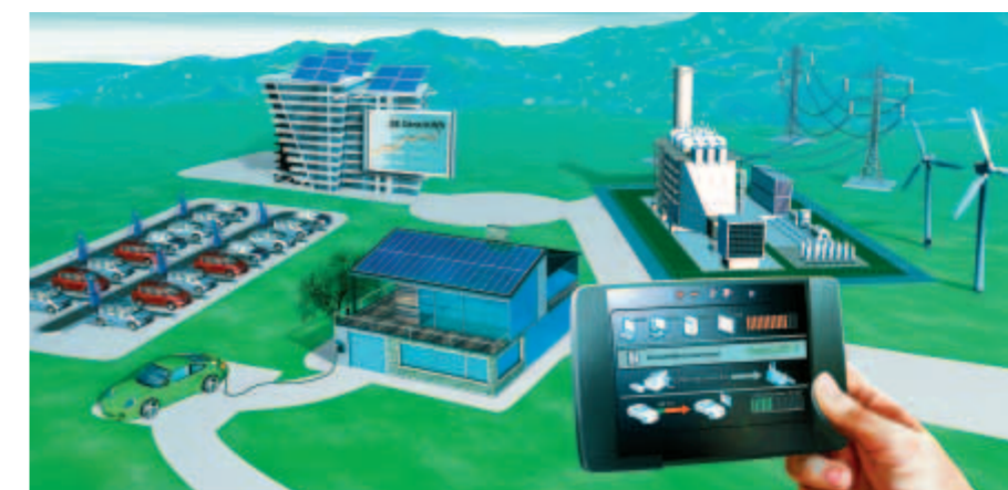
In the electricity supply of the future, various generators – including intermittent renewables – will provide power irrespective of demand, which will then partly have to be tailored to supply. Electric vehicles may be one practical way of storing excess power, since cars generally are in motion only 10 percent of the time. Our vehicles would then not only run on excess clean power, but also export power back to the grid in case of shortfalls. Consumers will also have consoles to control their systems.
