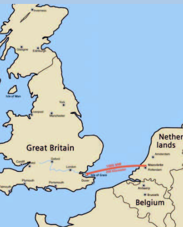
The new BritNed HVDC transmission system, designed and installed by Siemens, connects converter stations on the Isle of Grain in Kent in southeastern England and in Maasvlakte near Rotterdam.
