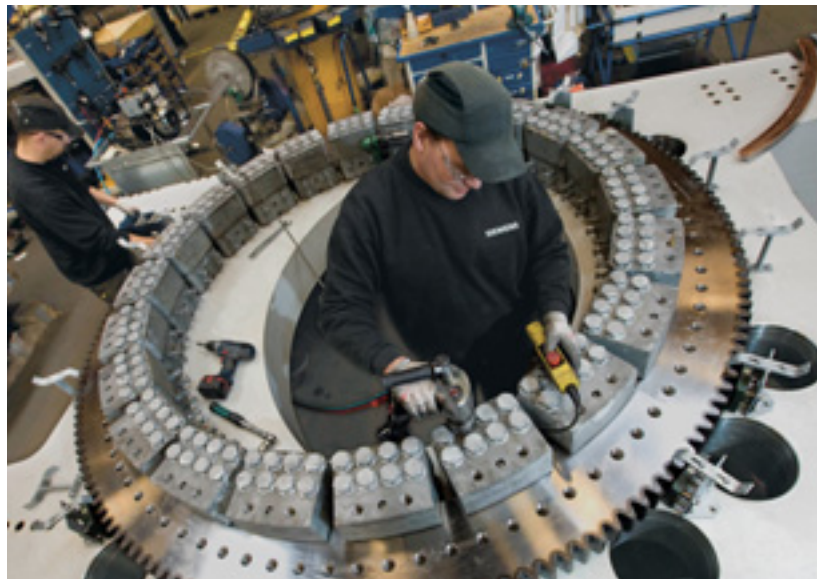
The yaw assembly area. Attention to quality and workmanship form the foundation for the reliability of Siemens wind turbines
