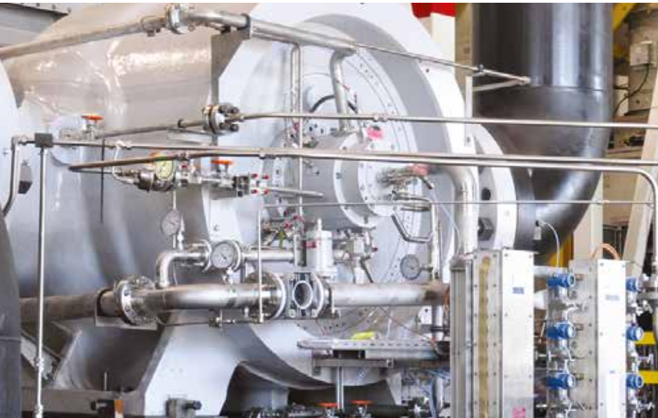
String test performed on Industrial RFBB36
