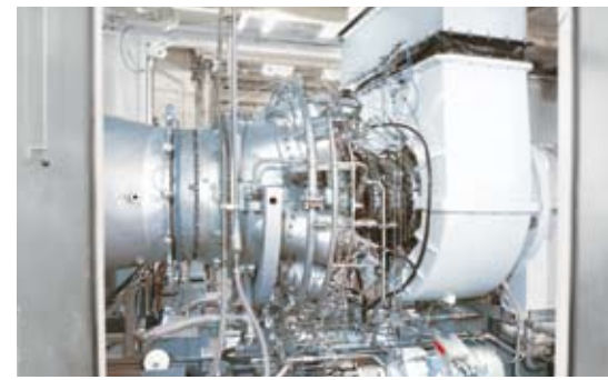
SGT-300 core engine test facility.
