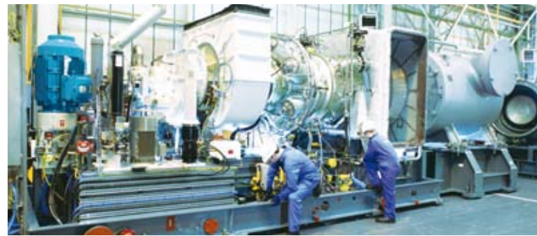
SGT-400 compressor package assembly.
