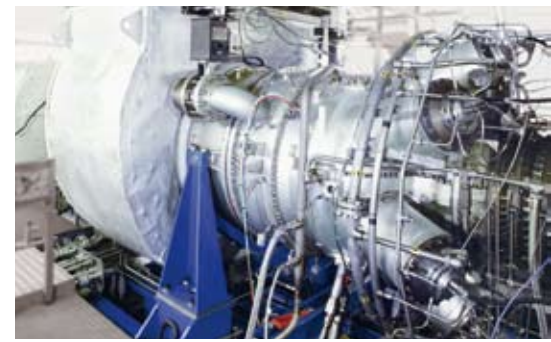
SGT-400 core engine test facility.
