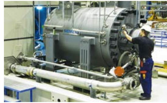
Compressor driven by SGT-700.
