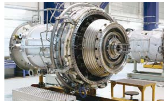
SGT-700 gas generator.
