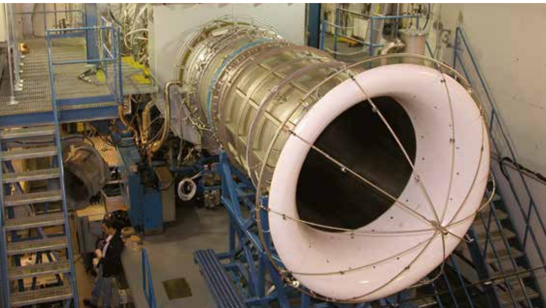
The Industrial Trent 60 engine on a test bed in Montreal, Canada
