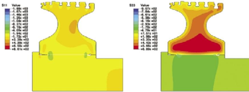
Fig 10. Non-linear fracture mechanics analysis for hypothetical worst-case scenarios
