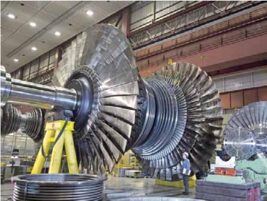
creases sharply over the length of the blade. The last three standardised blades have the main advantages of guaranteed vibration frequencies with a wide margin between the natural frequency at rated speed and resonance. The moving blades are locked in place by means of curved 'fir-tree' roots.
