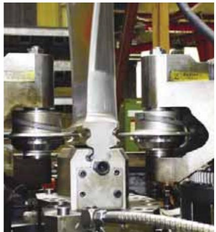
Fig 13. Rolling of LP blade root radii
