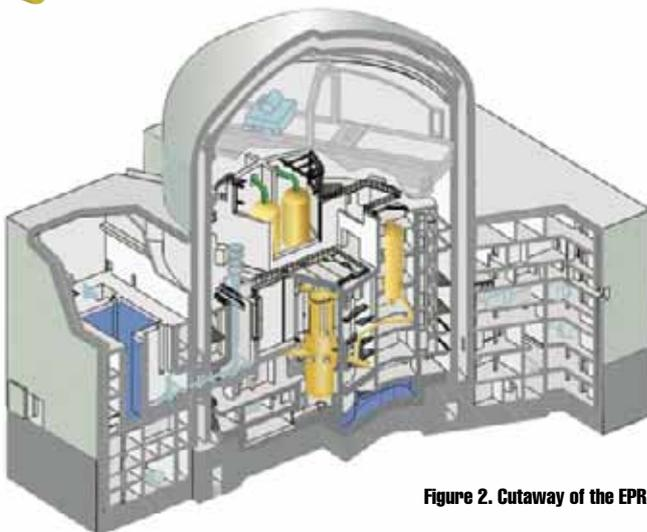
Figure 2. Cutaway of the EPR
