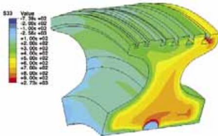
Fig 11. Residual compressive stress area after water spraying of disks
