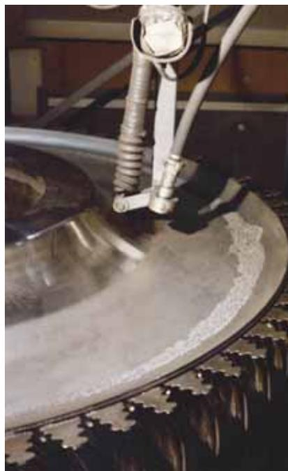
Fig 12. Shot peening of disk web area
