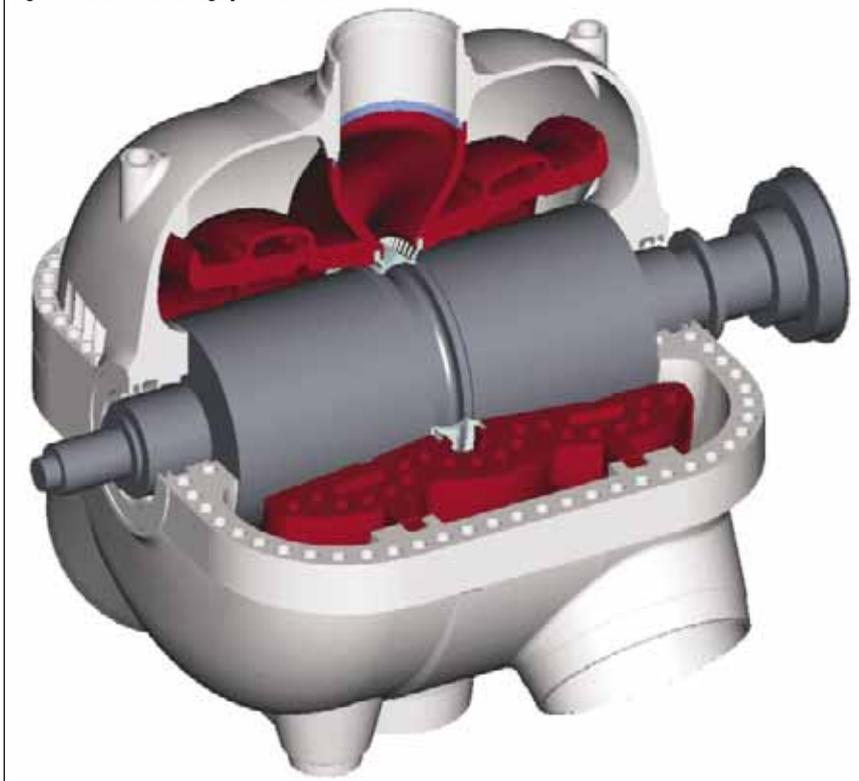
Fig 4. Longitudinal section of LP turbine
