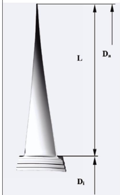
**Hub diameter  $D_i$  - 3060 mm, tip diameter  $D_a$  - 6720 mm, blade length  $L$  - 1830mm, blade weight (including root) - 340kg.**
