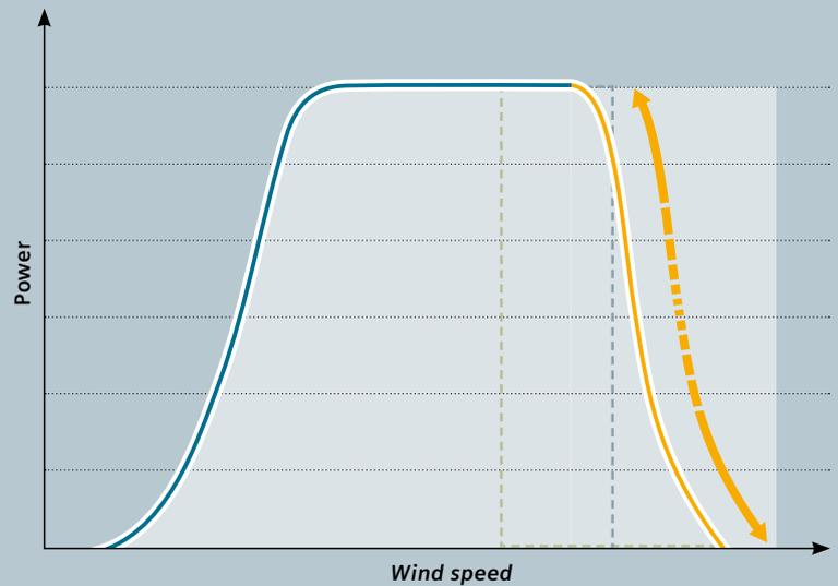
The orange line shows the extension in operation at high wind speeds
