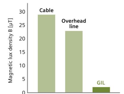
A comparison of the magnetic fields for different high-voltage transmission systems for a 400-kV double system at 2 x 1,000 MVA load.
