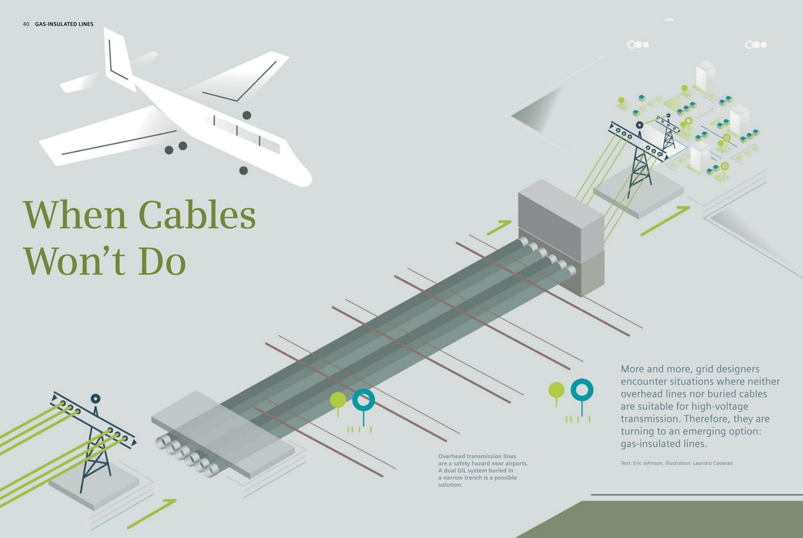
Overhead transmission lines are a safety hazard near airports. A dual GIL system buried in a narrow trench is a possible solution.
