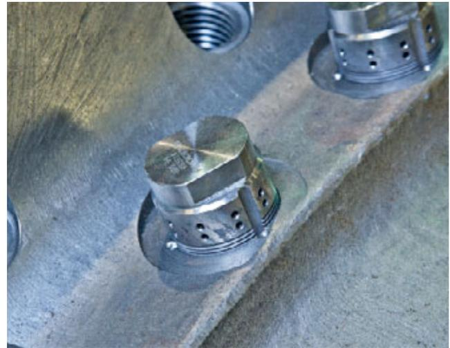
Fig. 5: Cooling air throttle in vane 2 section
