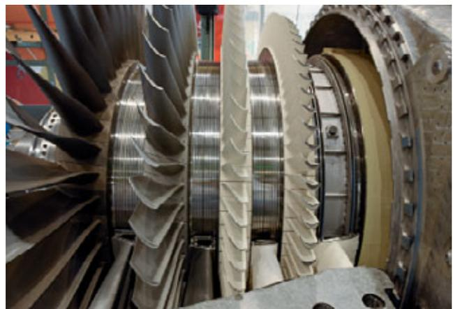
Fig. 3: Si3D blades on turbine stages 1 and 2
