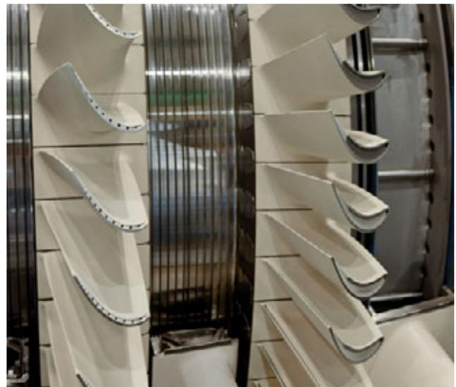
Fig. 6: Si3D blades and vanes on turbine stages 1 and 2
