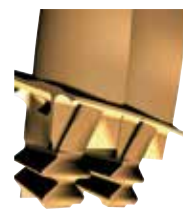
Two lobe axial cut serrations provide improved fatigue resistance
