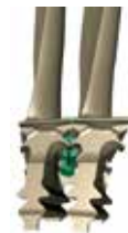
HP turbine blade under-platform damper to reduce aerofoil vibratory stresses and fatigue damage
