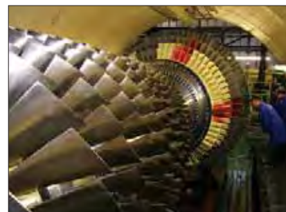
Figure 5. SGT5-8000H – axial 13-stage compressor.
